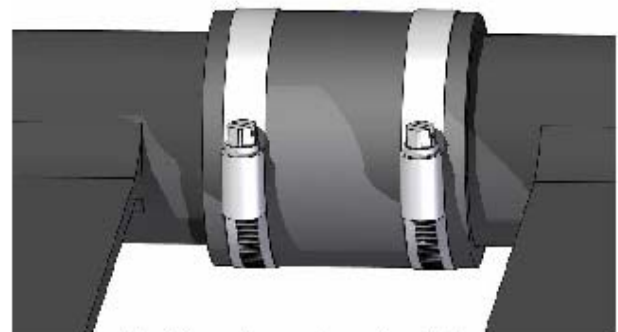
5. Rubber Coupling Installed
